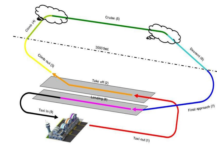
In TIER 1 the emission factors have been averaged over all flying phases assuming 10% of the fuel is used in the LTO. The emissions produced by aviation come from the use of jet fuel (jet kerosene and jet gasoline) and aviation gasoline (small piston engine aircraft only) the principal pollutants (common to other combustion activities)
