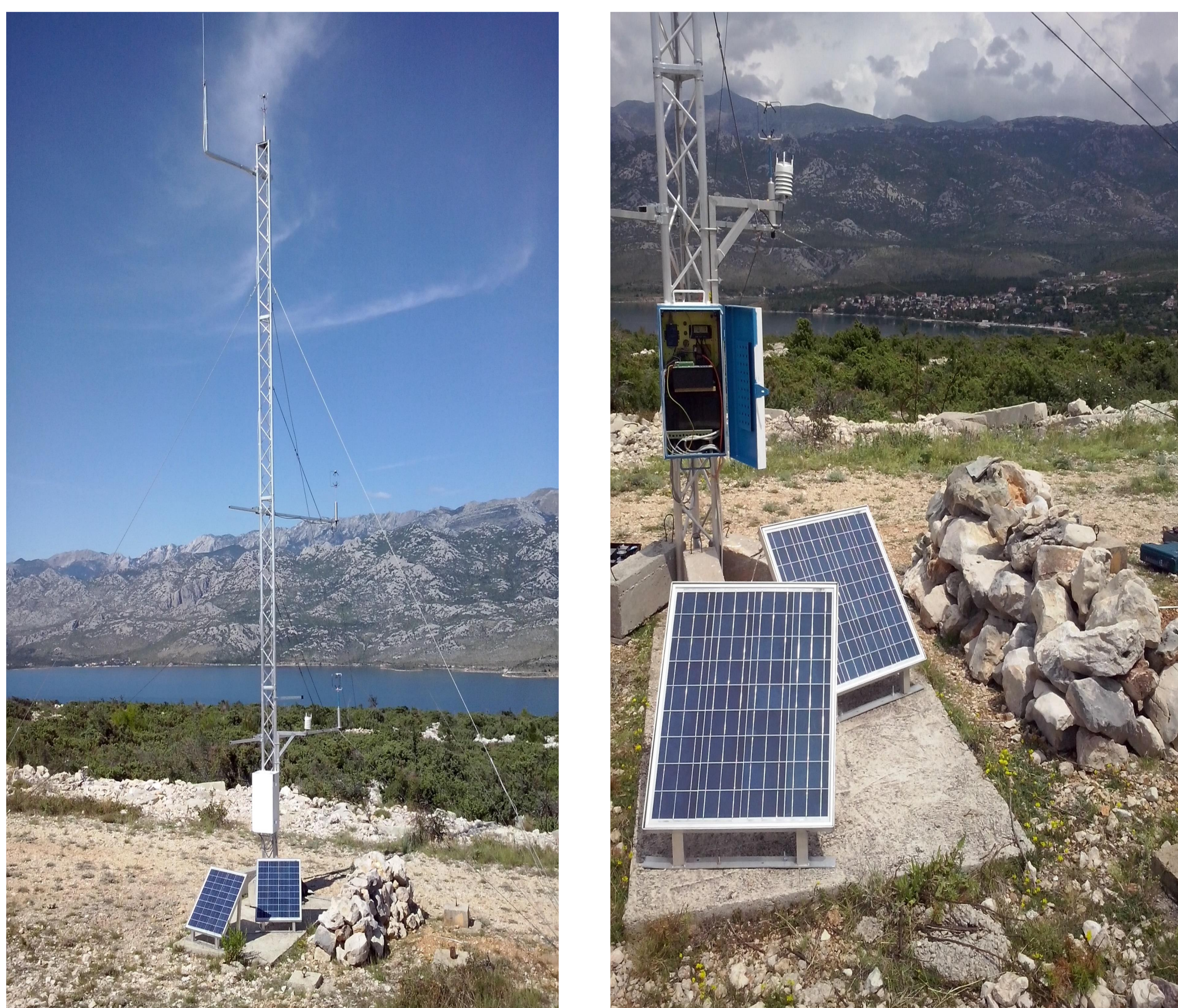
Figure 2. Left: Photo of assembled tower. Ultrasonic anemometers are mounted at 2, 5 and 10 m levels. Right: A photo of the tower base with solar panels in the foreground. Frontal panel facing SW while back panel faces SE.
