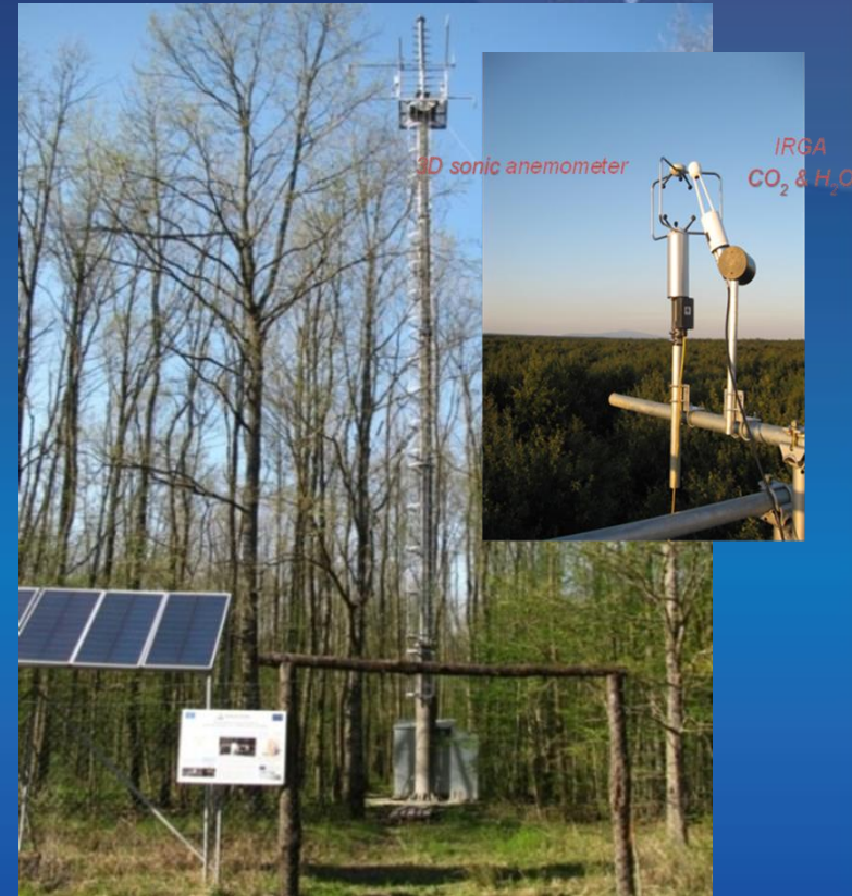
Figure 4. EC tower with instruments
